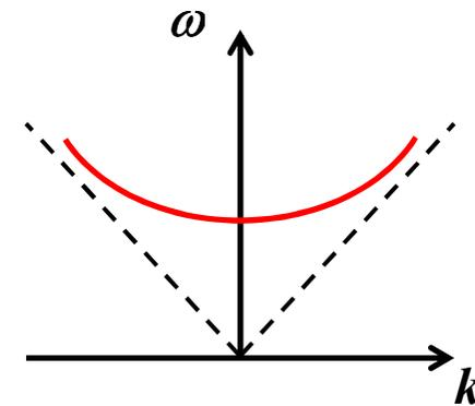
In order to be able to accelerate charged particles over any reasonable distance, the wave and the particle must have the same velocity. The waveguide is “loaded” with periodic structures to make this happen.
