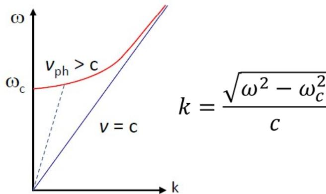
The phase velocity of a waveguide
