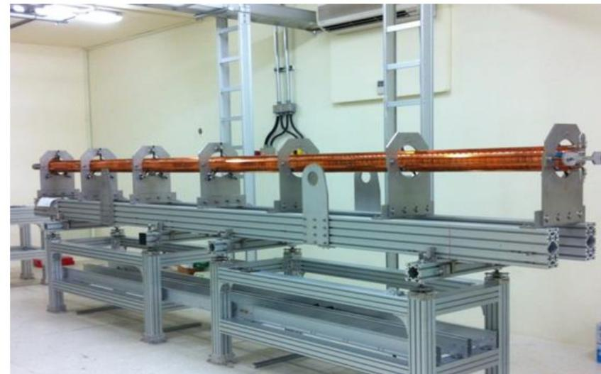
The 5.2 m constant gradient traveling wave linac structure
