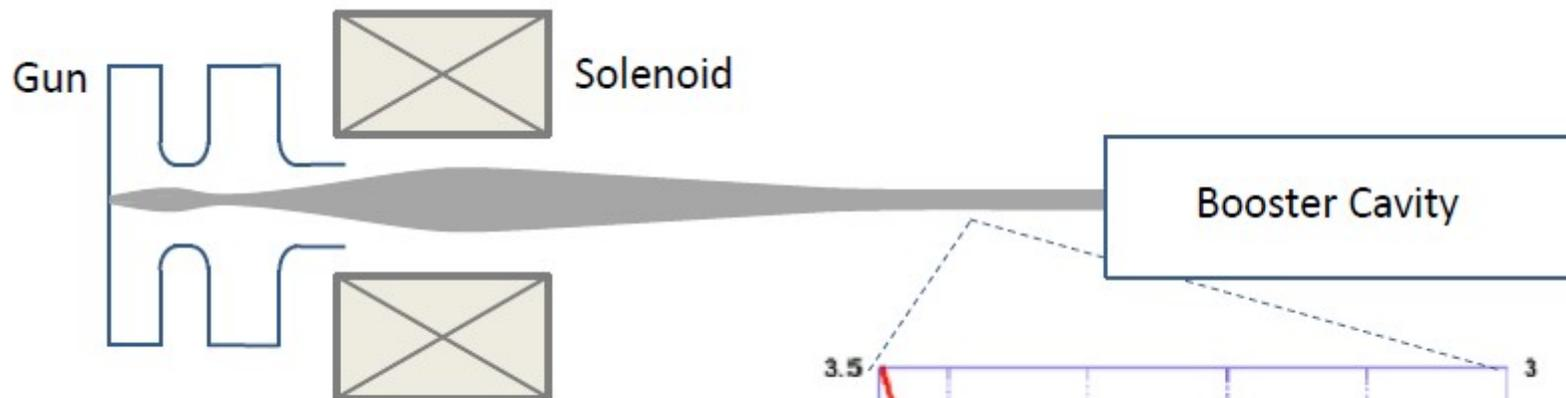
Emittance oscillations produce two emittance minima after the solenoid.
