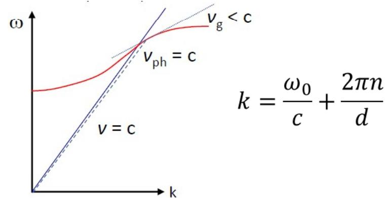
The phase velocity of a loading structure
