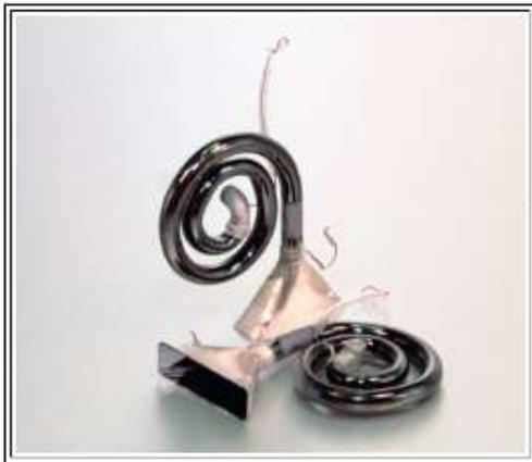
Fig. 8 Original CEMs made entirely of glass
