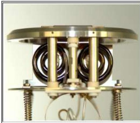
Fig. 9 CEM array before replacement
