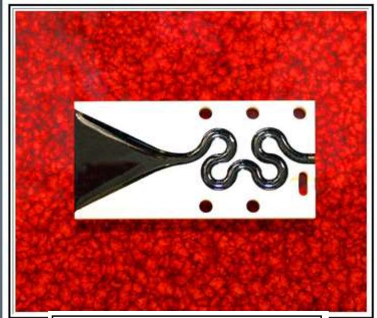
It's a detector responding to charged particles, hard and soft X-ray, and UV. Enhance  $10^8$  with  $\sim 2.5\text{KV}$  applied. FWHM = 8 ns.
