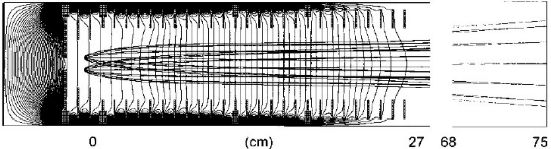
FIG. 1. Computer simulation of the ion optics. The potential contour spacing is 19.6 V/cm at 1000 V ion optics voltage. The ion trajectories shown correspond to ions with 1.2 eV initial kinetic energy sampled every  $30^\circ$ . The two ion born positions are separated by 10 mm. The pitch of the electrode plates was designed to be 1 cm.
