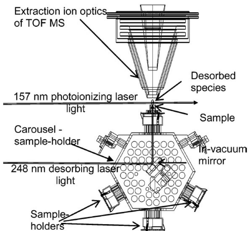
**Figure 1.** Schematic drawing of the experimental setup.
