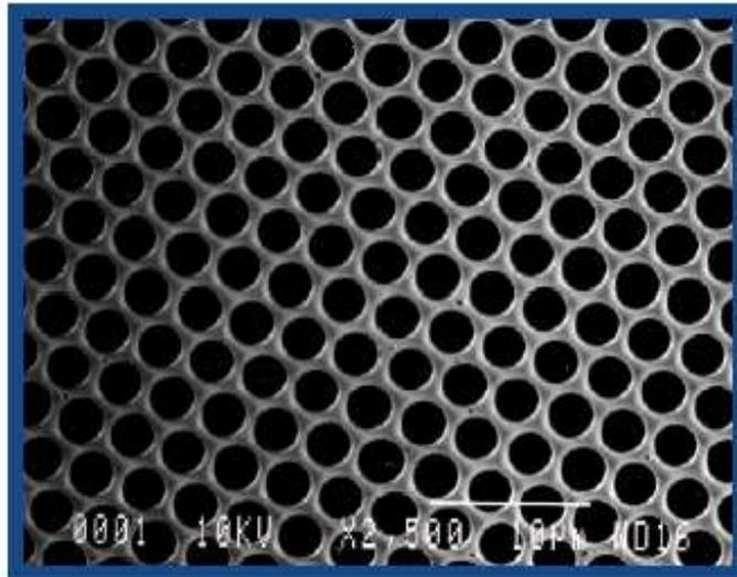
BURLE's 2-micron pore MCP provides the highest resolution in the world.
