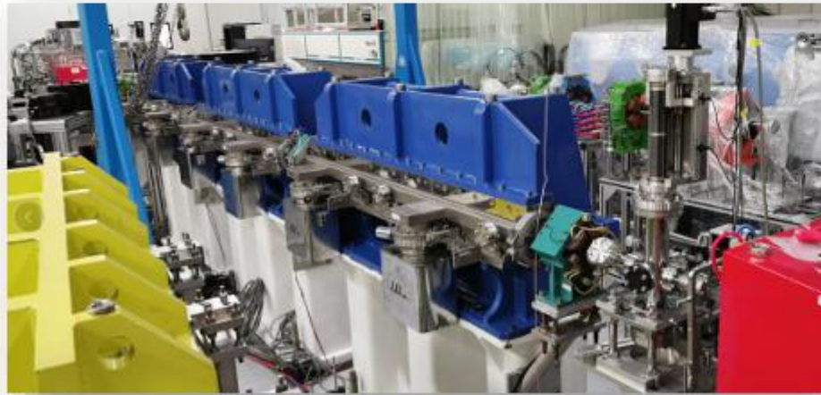
Three undulators with each length of 1.5 m
