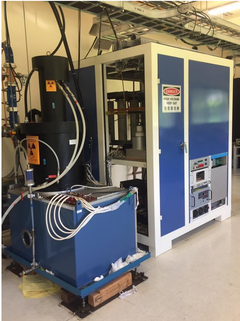
The Thales TH2100A in focusing magnet with X-ray shielding. The background is a 80 MW home-made line-type modulator.
