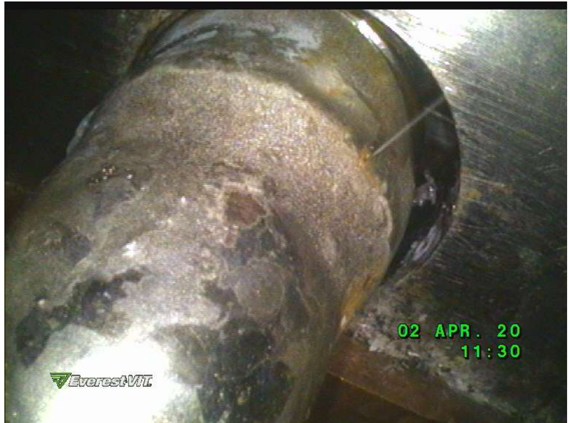
Leak was repaired by flame-brazing, unfortunately, several other leaks were found and had to be brazed
